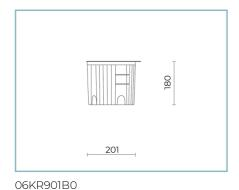
B132 Drive over recessed housing made of polypropylene. Colour: black RAL9005.
